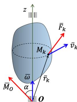
$$d'A(\bar{F}_k) = \bar{F}_k \bar{v}_k dt = \bar{F}_k (\bar{\omega} \times \bar{r}_k) dt = \bar{\omega} (\bar{r}_k \times \bar{F}_k) dt =$$
