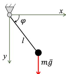
$$Q_\varphi = (mg)_x \cdot \frac{\partial x}{\partial \varphi} + (mg)_y \cdot \frac{\partial y}{\partial \varphi}$$
