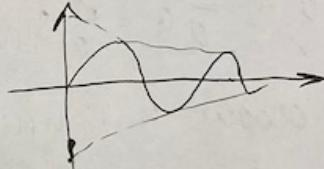
$$q = e^{-nt} (C_1 \cos \omega_1 t + C_2 \sin \omega_1 t)$$
