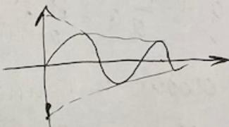
$$q = e^{-nt} (C_1 \cos \omega t + C_2 \sin \omega t)$$
