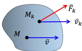
$$d'A(\bar{F}_k) = \bar{F}_k \bar{v}_k dt = \bar{F}_k \bar{v} dt = \bar{F}_k d\bar{r}$$
