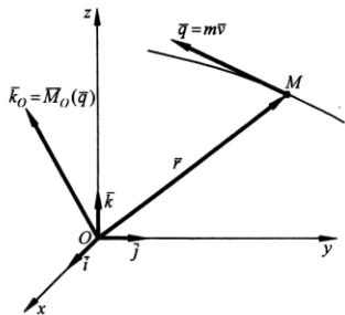
$$\bar{k}_0 = \bar{M}_O(\bar{q}) = \bar{r} \times \bar{q} = \bar{r} \times m\bar{v}$$
