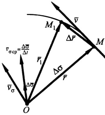
$$\bar{v}_\sigma = \lim_{\Delta t \rightarrow 0} \frac{\Delta \bar{v}}{\Delta t} = \frac{1}{2} \lim_{\Delta t \rightarrow 0} \left( \bar{r} \times \frac{\Delta \bar{r}}{\Delta t} \right) = \frac{1}{2} (\bar{r} \times \bar{v}) = \frac{1}{2} \bar{M}_O(\bar{v}), \quad (15.69)$$
