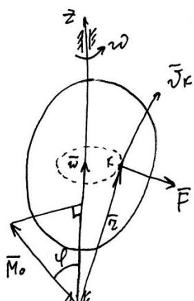
$$\begin{aligned} dA &= \bar{F} \bar{v} \, dt \\ \bar{v} &= \bar{\omega} \times \bar{r} - \varphi \omega \bar{r} \text{ вправо} \\ dA &= \bar{F} (\bar{\omega} \times \bar{r}) \, dt = \bar{\omega} (\underbrace{\bar{r} \times \bar{F}}_{\bar{M}_o(\bar{F})}) \, dt = \\ &= \bar{\omega} \bar{M}_o(\bar{F}) \, dt = \omega M_o \cos \varphi \, dt = \\ &= \underbrace{\omega \, dt}_{d\varphi} \cdot \underbrace{M_o \cos \varphi}_{M_z(\bar{F})} \end{aligned}$$
