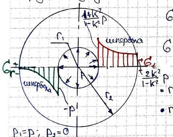
$$\sigma_r = -\frac{P r_1^2}{r_2^2 - r_1^2} + \frac{P \cdot r_1^2 r_2^2}{(r_2^2 - r_1^2) r^2}; \quad K = \frac{r_1}{r_2}$$
