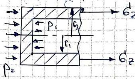
$$\sum z_i = 0: \sigma_z \pi (r_2^2 - r_1^2) = P_1 \pi r_1^2 - P_2 \pi r_2^2$$
