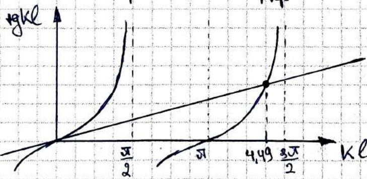
$$kl = 4.49 \Rightarrow k = \frac{4.49}{l} \Rightarrow \sqrt{\frac{F_{kp}}{E J_{min}}} = \frac{4.49}{l} \Rightarrow F_{kp} = \frac{4.49^2 E J_{min}}{l} \Rightarrow F_{kp} = \frac{\pi^2 E J_{min}}{(0.7l)^2}$$
