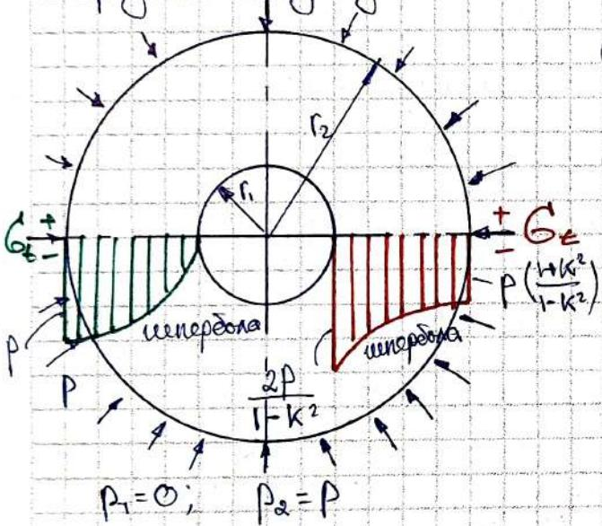
$$G_r = \frac{-P r_2^2}{r_2^2 - r_1^2} = \frac{(-P) \cdot r_1^2 r_2^2}{r_2^2 - r_1^2} \cdot \frac{1}{r_2^2} ; k = \frac{r_1}{r_2}$$
