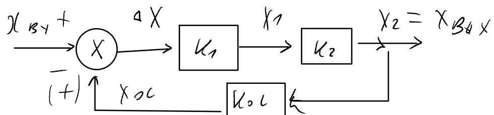
$$\left. \begin{array}{l} \Delta x = x_{Bx} (+) x_{oc} \\ x_1 = k_1 \Delta x \\ x_2 = k_2 x_1 = x_{B6x} \\ x_{oc} = k_{oc} x_2 = k_{oc} x_{B6x} \end{array} \right\} \Delta x - \text{это ошибка}$$
