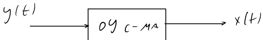
$$a_n \frac{d^n x}{dt^n} + \dots + a_0 x = b_m \frac{d^m y}{dt^m} + \dots + b_0 y$$
